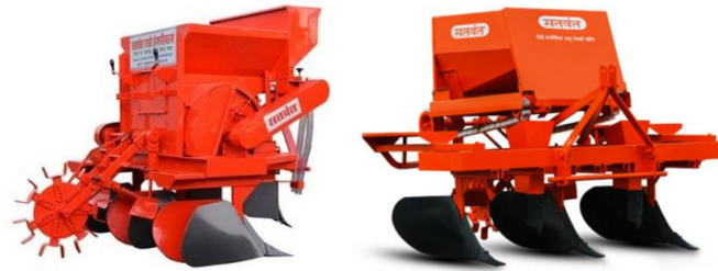
Fig. 1 (a)Tractor mounted automatic potato planter (b) Semi-automatic potato planter
