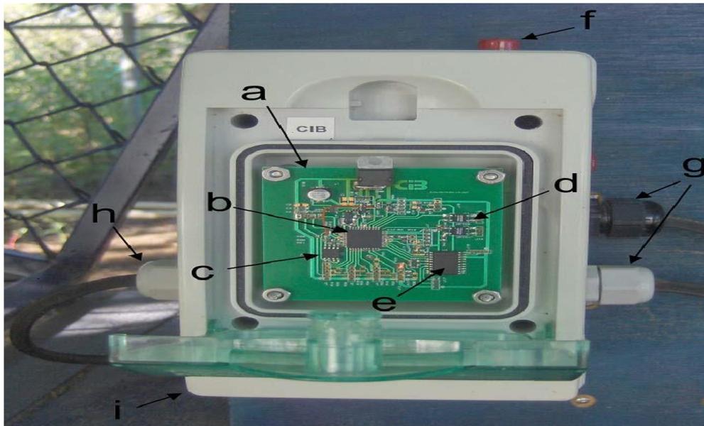
Fig. 2. WIU. (a) Electronic component PCB. (b) Master microcontroller. (c) Solid state memory. (d) Optical isolators. (e) RS-232 interface. (f) Push button. (g) Output cables to pumps. (h) Supply cable from charge controller. (i) PCV box. Source - Gutiérrez, et. Al. (2014)
