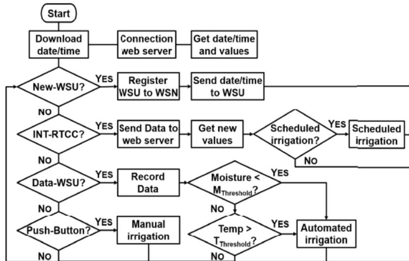
Fig. 3. Algorithm of the master microcontroller in the WIU for the automated irrigation system. Source - Gutiérrez, et. Al. (2014)
