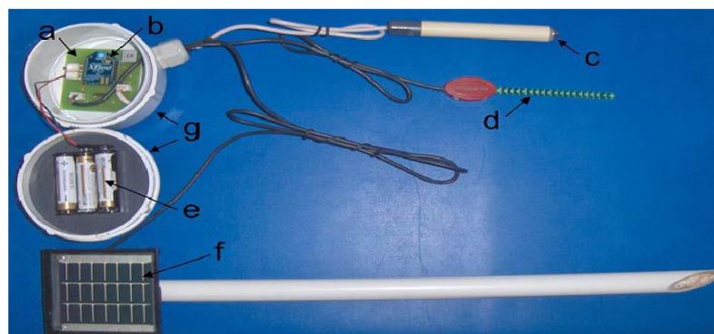
Fig. 1. WSU. (a) Electronic component PCB. (b) Radio modem ZigBee. (c) Temperature sensor. (d) Moisture sensor. (e) Rechargeable batteries. (f) Photovoltaic cell. (g) Polyvinyl chloride container. Source - Gutiérrez, et. Al. (2014)
